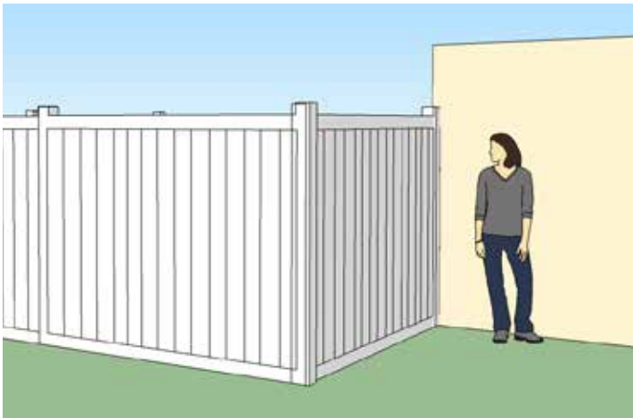
The illustration above shows proper placement of a fence at the back corner of the residence. In this case, the residence is on an interior lot, so the fence can be located at the property line.
